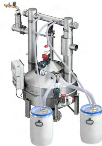
Lipator-S-RA: Grease separator for partial disposal, for automated grease/sludge extraction
